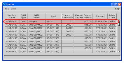
4 Double-click the QAM you want to modify to open the Set Up QAM window.
