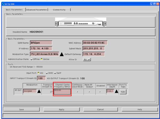
5 Record the Channel Center Frequency (output frequency). You will need this value later, when you restore the output frequency on the BFS QAM.
