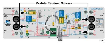
4 Remove the RF amplifier module from the housing.
