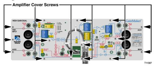
2 Remove the four (4) Diplex filters using the plastic handle on the component. There are two (2) "mirrored"/blue PCB material and two (2) "non-mirrored"/green PCB material Diplex filters.
