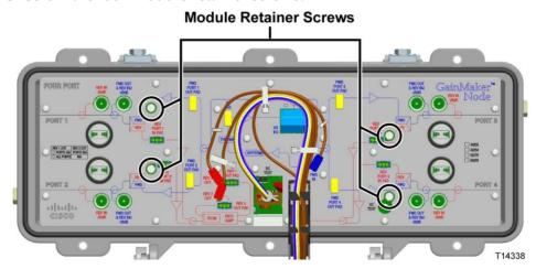
4 Remove the RF amplifier module from the housing.
