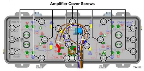
2 Remove the four (4) Diplex filters using the plastic handle on the component.
