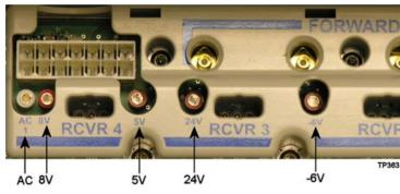
**Note:** OIBs with the shorting condition will indicate improper voltages at the test points. Typically, only the 5 V DC is affected by the shorting condition.
