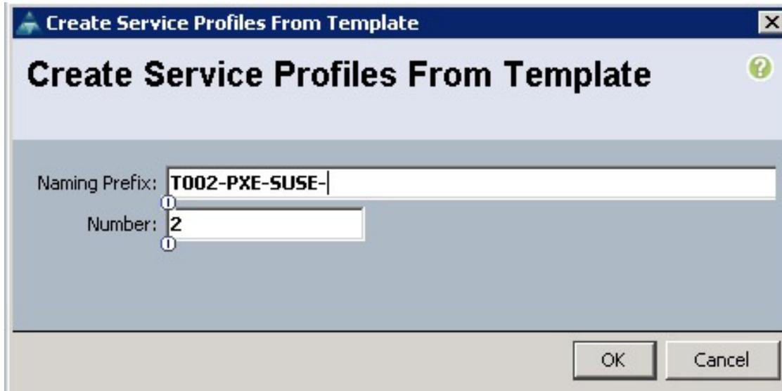
3 The service profiles are created. Verify them in the Service Profiles tree. The MAC addresses created are important in configuring the PXE boot. You can find them in the created service profile in the Networking section. Note the MAC addresses of both adapters for future reference.
