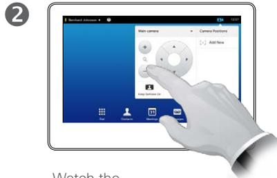
Watch the screen of your video system while using the camera's pan tilt and zoom, if needed.
