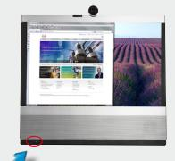
To start the system again, press the **Power** button until the LED illuminates (green light).
