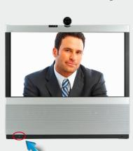
To start the system again, press the **Power** button until the LED illuminates (green light).
