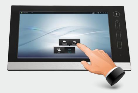
The EX90 can be configured via the touch screen controller or via its web interface. For full access to all configurable parameters the web interface must be used—the touch screen controller provides access to a limited set of parameters only.
