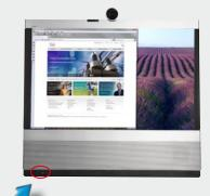
To start the system again, press the **Power** button until the LED illuminates (green light).
