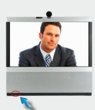
To start the system again, press the **Power** button until the LED illuminates (green light).
