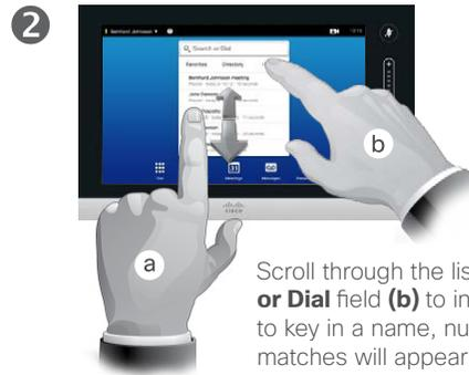
Scroll through the list **(a)**, or tap the **Search or Dial** field **(b)** to invoke the virtual keyboard to key in a name, number or address. Possible matches will appear as you type.
