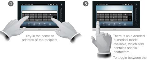
alphanumerical mode and the extended numerical mode tap the key in the lower left corner of the keyboard, as outlined.
