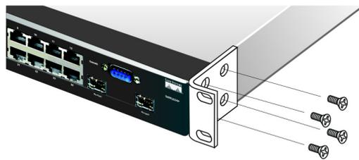
3. Make sure the brackets are properly attached to the switch.
