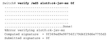
To display the contents of the Flash memory, enter the **show flash** command. The Flash contents listing does not include the checksum of the individual files. To recompute and verify the image checksum after the image has been copied into the Flash memory, enter the **verify** command.
