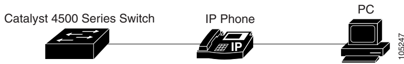
Figure 29-1 Cisco 7960 IP Phone Connected to a Catalyst 4500 Series Switch
