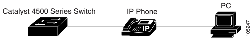
Figure 30-1 Cisco 7960 IP Phone Connected to a Catalyst 4500 Series Switch
