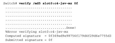
To display the contents of the flash memory, enter the **show flash** command. The flash contents listing does not include the checksum of the individual files. To recompute and verify the image checksum after the image has been copied into the flash memory, enter the **verify** command.
