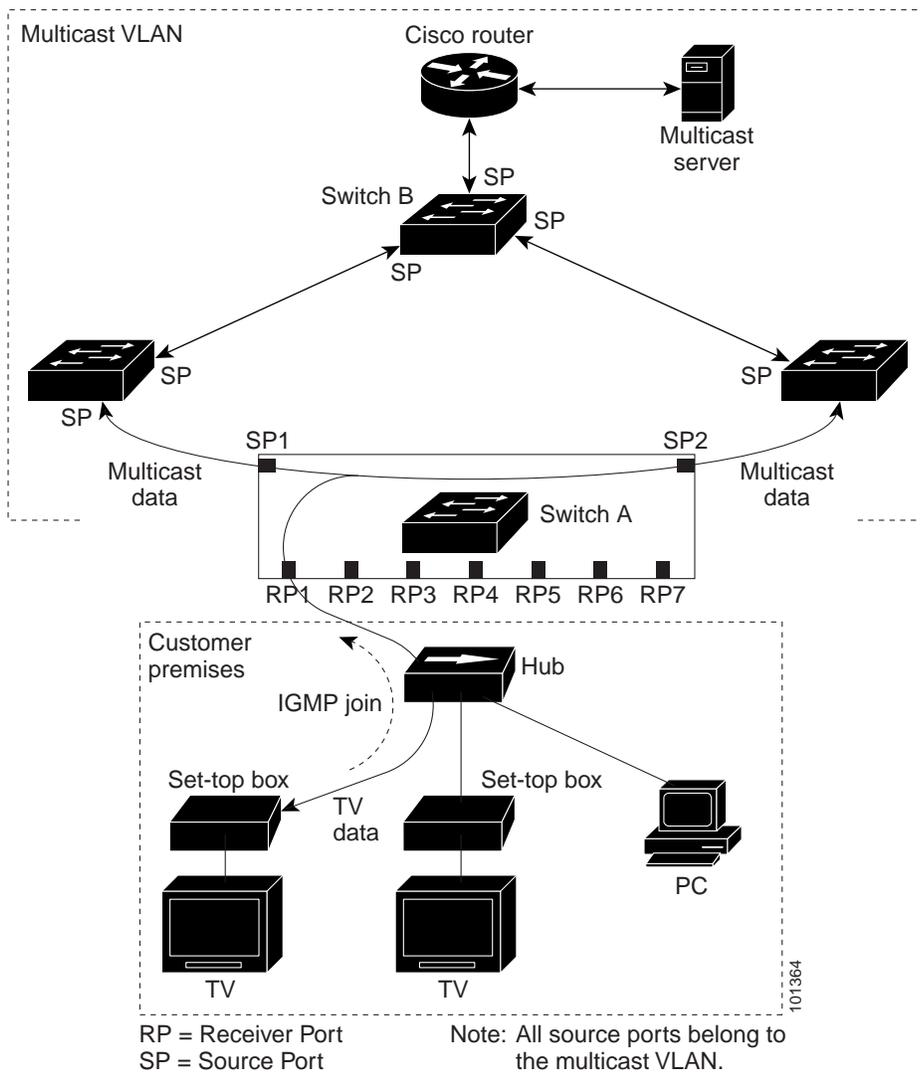
When a subscriber changes channels or turns off the television, the set-top box sends an IGMP leave message for the multicast stream. The switch CPU sends a MAC-based general query through the receiver port VLAN. If there is another set-top box in the VLAN still subscribing to this group, that set-top box must respond within the maximum response time specified in the query. If the CPU does not receive a response, it eliminates the receiver port as a forwarding destination for this group.
