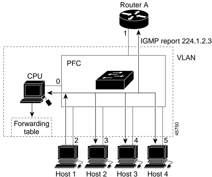
Router A sends a general query to the switch, which forwards the query to ports 2 through 5, which are all members of the same VLAN. Host 1 wants to join multicast group 224.1.2.3 and multicasts an IGMP membership report (IGMP join message) to the group. The switch CPU uses the information in the IGMP report to set up a forwarding-table entry, as shown in [Table 24-1](#), that includes the port numbers connected to Host 1 and the router.
