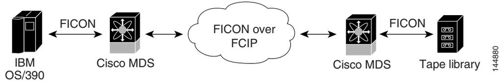
**Figure 12-6 Host Accessing Standalone IBM-VTS (Virtual Tape Server) /STK-VSM (Virtual Shared Memory)**
