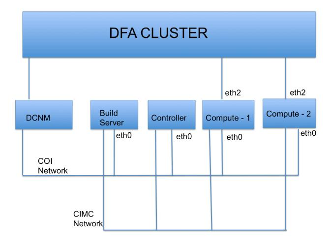
Ensure that all the UCS' are connected to each other. The sample topology has the build server, the controller and the computes connected through eth0. This is referred as the COI network.
