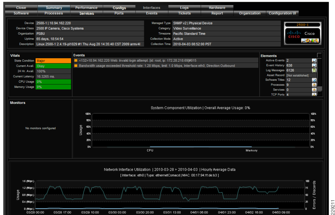
Figure 7-13 PSS Faults—Component Summary View (Cisco IP Camera)
