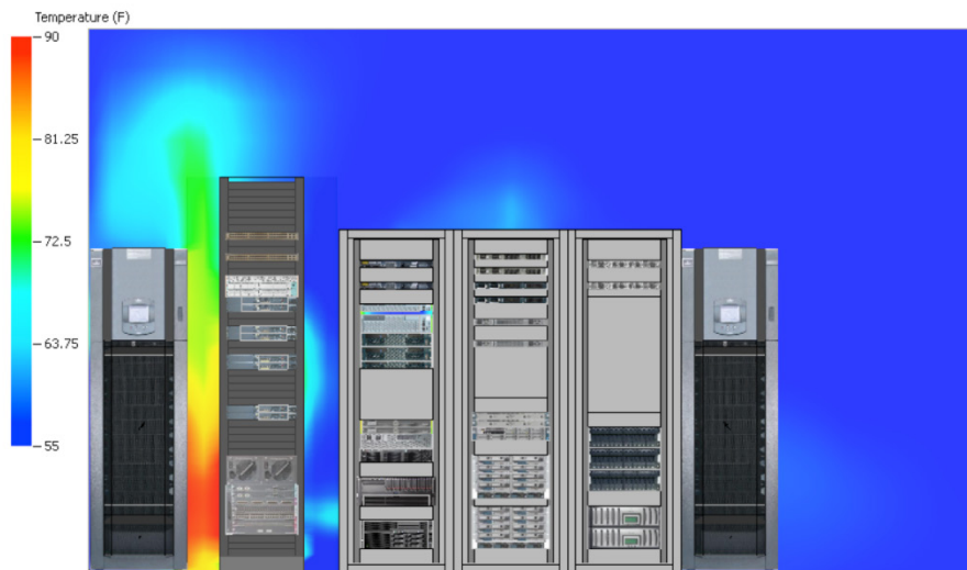
Figure 23 - Cross-sectional view of R1 temperature distribution through the centerline of the rack
