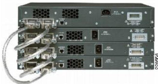
Figure 3-6 Cisco Catalyst 3750G StackWise Cabling
