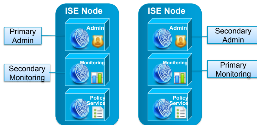
Figure A2 A Simple, 2-Node Distributed ISE Deployment for Redundancy
