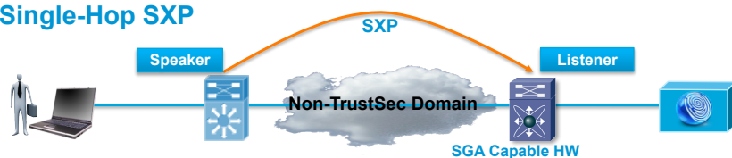
Figure 31: Single-Hop vs. Multi-Hop SXP Connections
