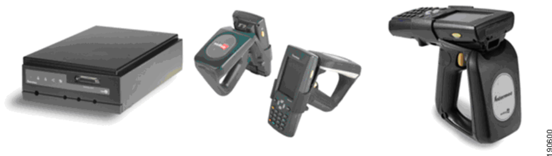
Figure 6-16 Portable RFID Interrogators with Integrated Wi-Fi Uplink
