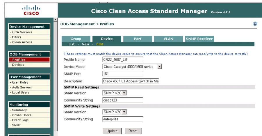
Switch Configuration for SNMP
