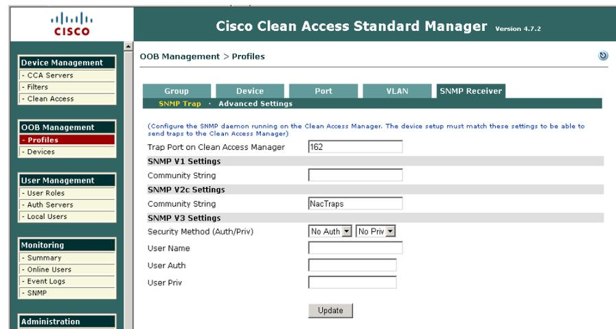
The switch needs to be configured to enable SNMP traps to be sent to the NAC Manager. In addition, it is recommended to increase the default switch CAM table entry flush timer to 1 hour per Cisco best practice recommendations for NAC OOB. This reduces the
