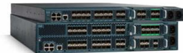
Figure 2. Cisco UCS 6120XP 20-Port Fabric Interconnect (Top) and Cisco UCS 6140XP 40-Port Fabric Interconnect
