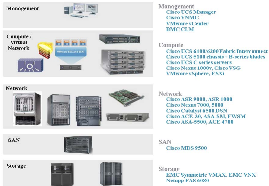
Figure 2-1 VMDC Infrastructure Components
