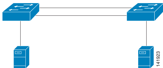
Figure 5-24 Logical EtherChannel Over EoMPLS
