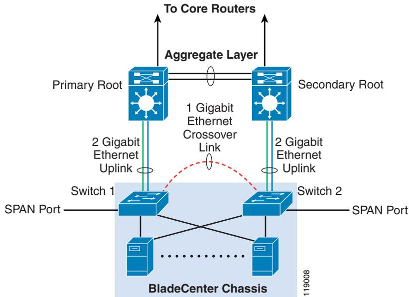
The disadvantage in these topologies is that in the event of device or link failures external to the BladeCenter, the redundant traffic path uses lower bandwidth links. You must monitor the link and device failures so you can quickly restore the higher bandwidth traffic path.
