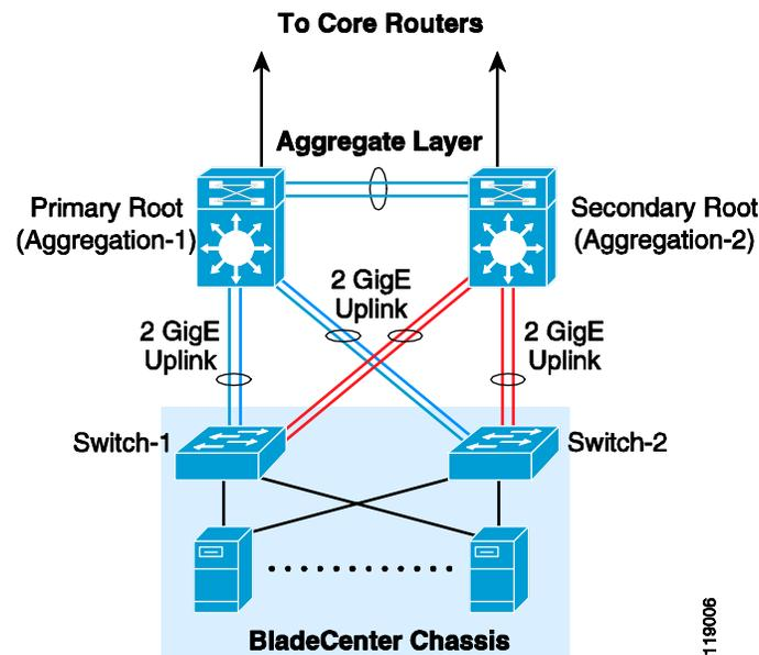
This provides a fully redundant topology, in which each BladeCenter switch has a primary and backup traffic path. Also notice that each Cisco IGESM switch has a deterministic topology in which RPVST+ provides a convergence time of less than one second after a failure. The environment is highly predictable because there is a single primary path used at all times, even when servers are dual-homed in active-standby scenarios.
