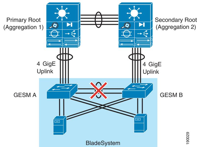
The inverted “U” design provides a highly available blade server environment using NIC teaming and Layer 2 trunk failover. The CGESM Trunk Failover feature disables downstream server ports when the uplink port channel fails. Disabling the downstream server ports of the CGESM allows a properly configured ProLiant blade server NIC team to converge traffic to the remaining active NICs homed to the other CGESM in the BladeSystem.
