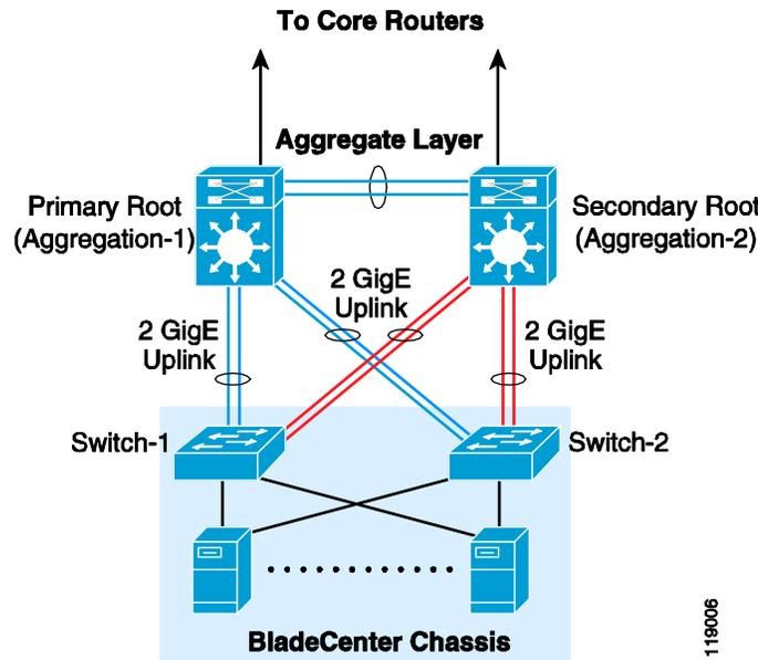
The recommendation is to use RPVST+ because it provides convergence of less than one second in case of device or link failures. In addition to rapid convergence, RPVST+ incorporates many enhanced Cisco Layer 2 features, including BackboneFast and UplinkFast, which are used by default when you enable RPVST+.
