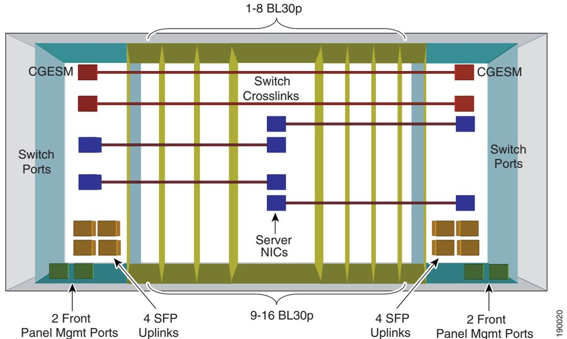
Each CGESM has four external SFP ports supporting 1000Base-SX and 10/100/1000Base-T on the rear of the enclosure and two external 10/100/1000Base-T ports on the front panel. These six ports provide connectivity to the data center or other external network. For more information, see the HP Blade Systems at the following URL:
