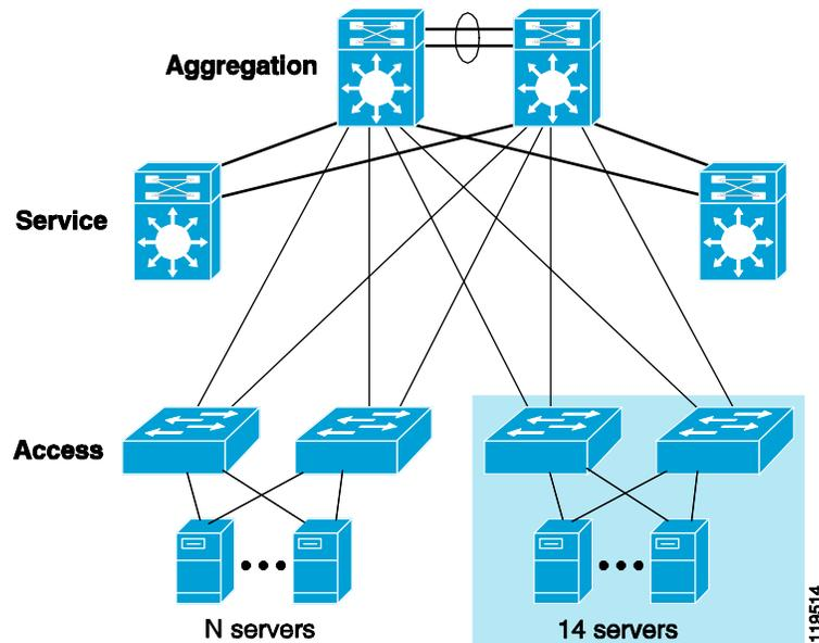
Blade servers, on the other hand, are connected to the integrated IGESMs, which are also connected to the aggregation switches. The slot gained by moving service modules to the service layer switches lets you increase the density of ports used for uplink connectivity.
