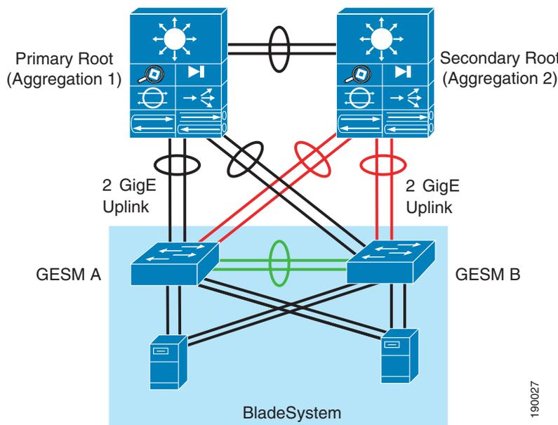
RPVST+ fulfills the high availability requirements of this design and is the recommended mode of spanning tree operation. RPVST+ provides fast convergence (less than one second) in device or uplink failure scenarios. In addition, RPVST+ offers enhanced Layer 2 features for the access layer with integrated capabilities equivalent to UplinkFast and BackboneFast.
