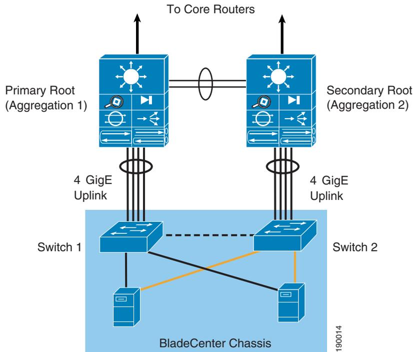
As noted with the previous design, a link failure between the BladeCenter switch and its associated aggregate switch isolates the blade server. The blade server is not aware of the network connectivity issues occurring beyond its own NIC. The trunk failover feature allows the Cisco IGESM and the blade server NIC teaming drivers to account for this scenario. The tests performed with this design achieved an average convergence of network traffic in three seconds.
