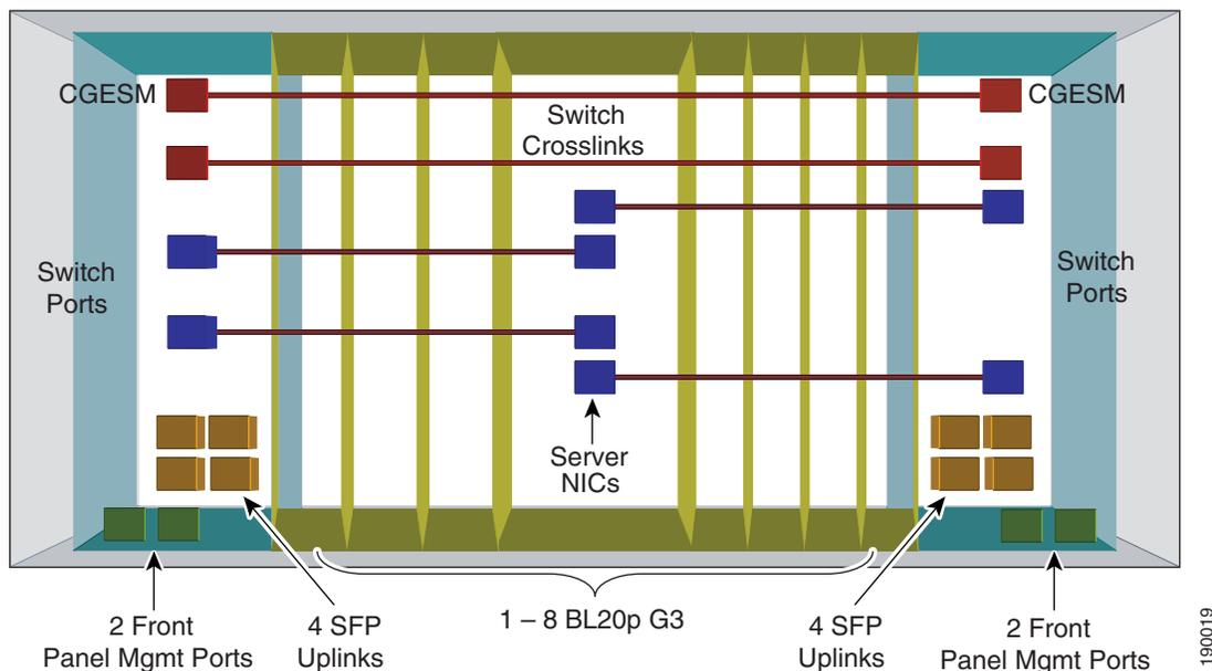
**Figure 2-18** HP BladeSystem p-Class Enclosure with Proliant BL30p Servers
