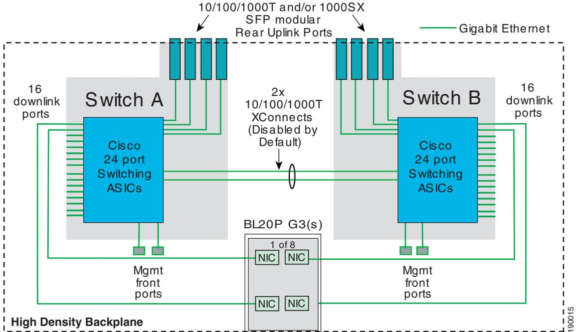
The HP BladeSystem p-Class backplane provides power and network connectivity to the blades. The interconnect bays house a pair of CGESMs, which provide a highly available and multi-homed environment where each server blade is Gigabit attached to each CGESM. Figure 2-14 illustrates how the HP BladeSystem p-Class logically provides Ethernet connectivity.
