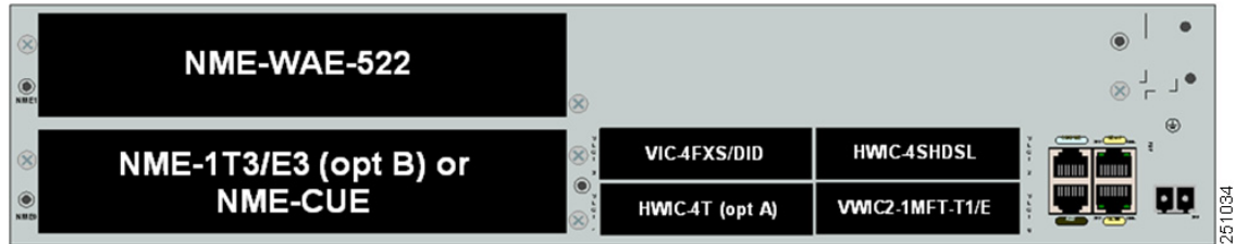
Figure 70 Interface Card and Service Module Configuration On a Cisco 3825
