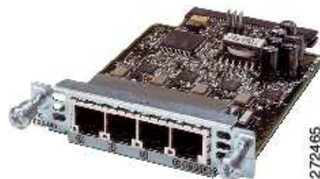
Figure 54 Four Port FXS/DID Voice Interface Card
