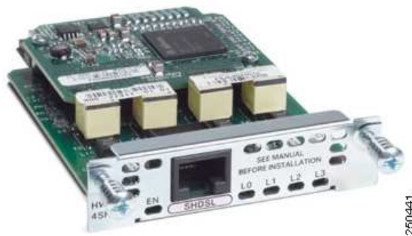
Figure 27 4-Port Symmetric High-Speed DSL (SHDSL) WAN Interface Card (HWIC-4SHDSL)
