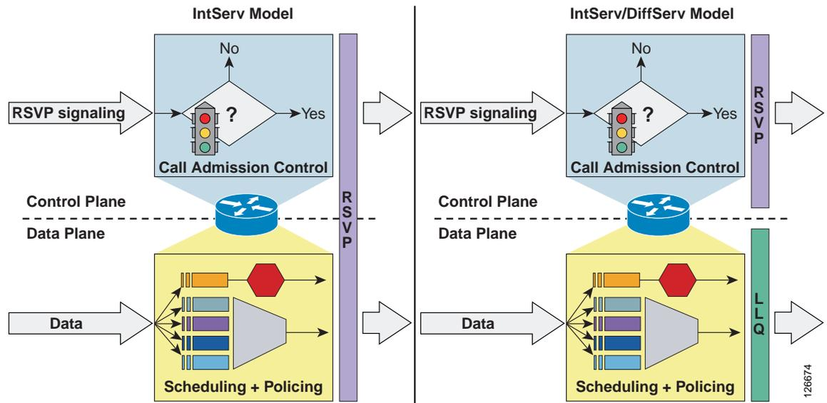
The Streamlined Medium Branch Network used the IntServ/DiffServ RSVP mechanism to control the number of calls placed on the network, but relied on the established QoS policy explained in the “[Quality of Service](#)” section on page 42 to control actual packet scheduling. This model is appropriate for the Streamlined Medium Branch Network because all LLQ-destined traffic is controlled by RSVP.
