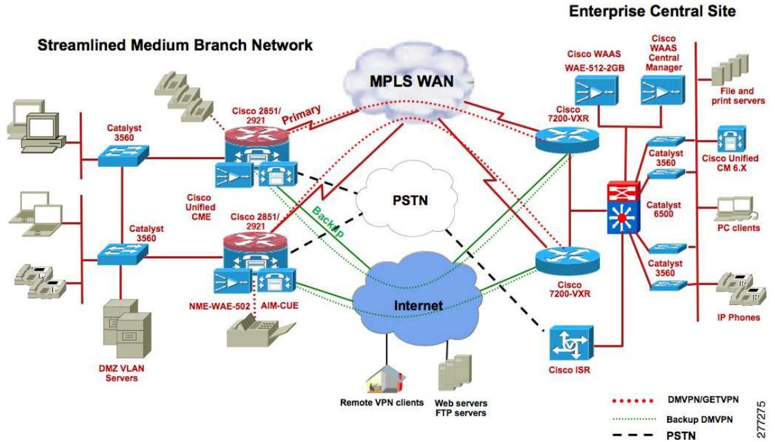
Figure 4 MPLS WAN, Cisco Unified SRST Mode
