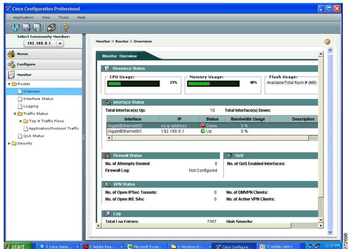
In monitor mode, Cisco Configuration Professional provides an overview of router status and performance metrics such as the Cisco IOS release number, interface status (up or down), and CPU and memory usage. The monitor mode also allows users to view the number of network access attempts that were denied by Cisco IOS Firewall, and provides easy access to the firewall log. Additionally, VPN status, such as the number of active IPsec tunnels, can be monitored.
