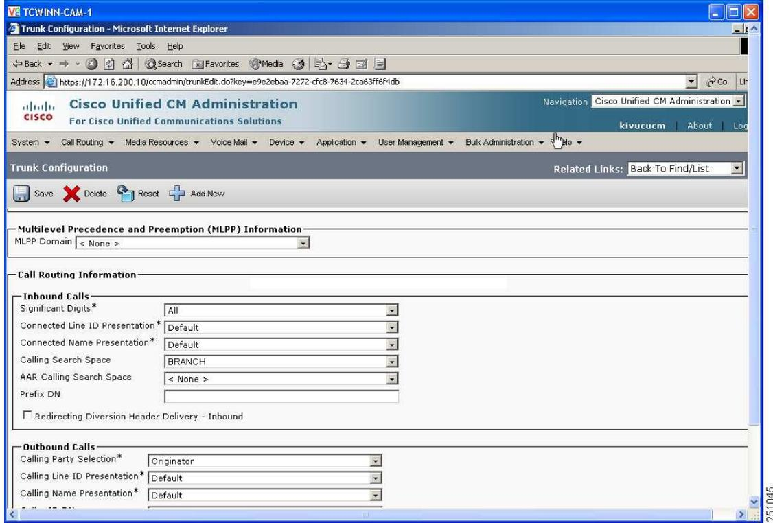
Figure 34 SIP Trunk Cisco Unified CM Configuration (3 of 3)
