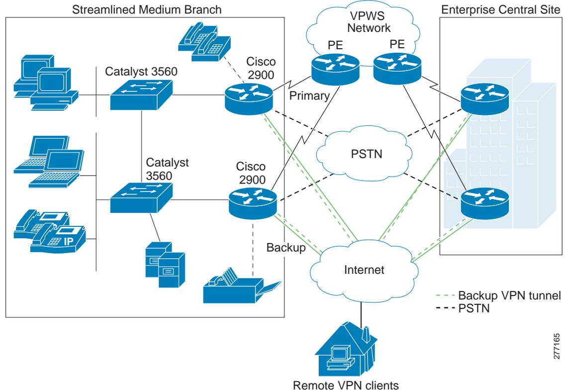
VPWS services allow the enterprise to keep its existing WAN infrastructure and to transparently connect to the service provider's Ethernet network, providing a transparent migration path to VPLS services. The leased-line connections to the PE device continue to use the typical Layer 2 encapsulation mechanism:
