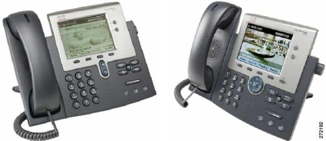
The Cisco Unified IP Phone 7962G GE and Cisco Unified IP Phone 7965G, shown in [Figure 8](#), were selected for the high call-volume use case. Both phones support the same features and differences as the Cisco Unified IP Phone 7942G and Cisco Unified IP Phone 7945G phones, and both phones support four additional phone lines.
