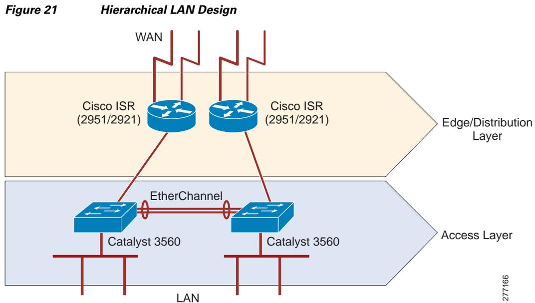
Switches must support many features to facilitate interoffice connectivity. Features of the Catalyst 3560 that were leveraged by the Streamlined Medium Branch Network are described in the following sections:
