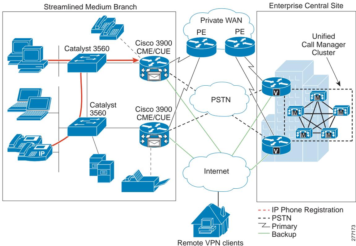
The local call control model eliminates dependency on out-of-the-branch control elements that would otherwise have to be accessed over the WAN. Thus, a WAN link failure has no effects on functionality provided by the IP telephony network; the network changes only the path over which the external WAN calls are routed.
