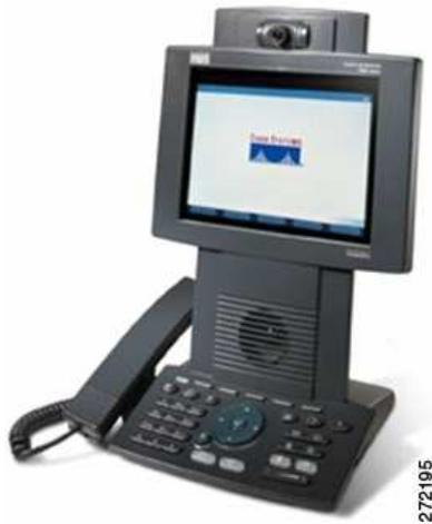
The Cisco Unified IP Conference Station 7936, shown in [Figure 11](#), was selected for the conference room scenario. The conference station offers a regular telephone keypad plus three soft keys, menu navigation keys, and a backlit, pixel-based LCD display.
