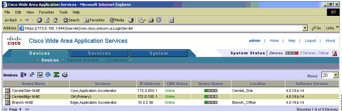
For ease of use and to start collecting statistics earlier, you need to change a few parameters. In the following steps, you extend the central manager session timeout interval and modify the intervals by which the Cisco WAAS central manager or Cisco WAE pulls or pushes data to and from the Cisco WAAS Central Manager.
