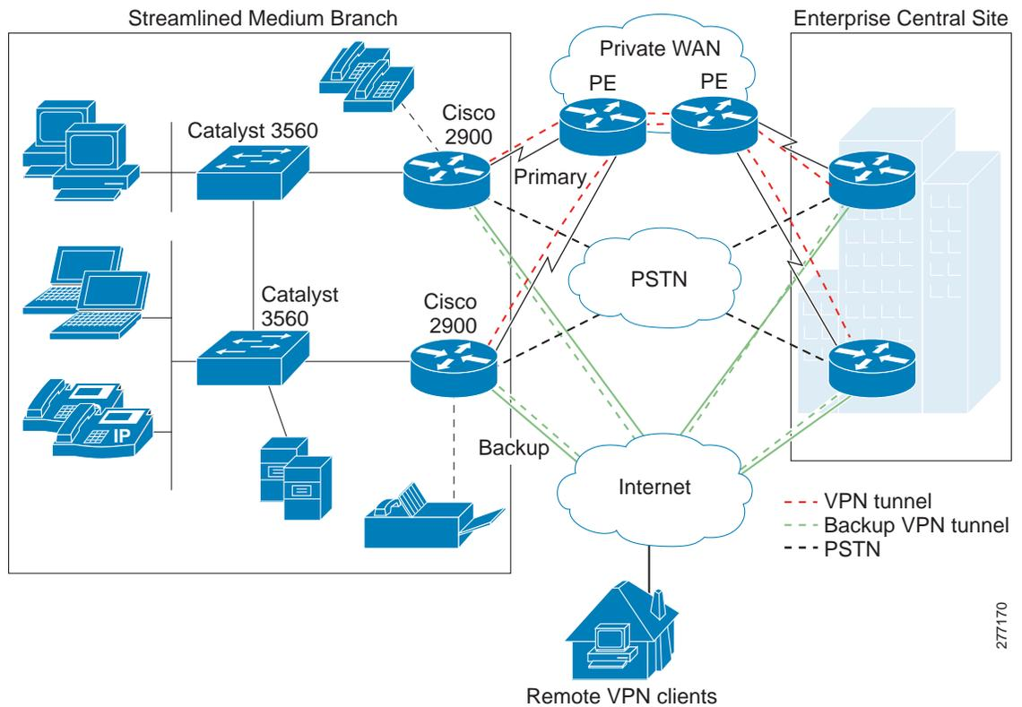
IP-based WAN VPNs routed over the Internet have in recent years become an attractive alternative to traditional Layer 2 WAN deployments. IP VPNs offer low cost, secure, flexible, and scalable site-to-site connectivity. There are a number of WAN VPN options, and selecting the appropriate one involves many considerations. For a branch office the most important of these considerations are:
