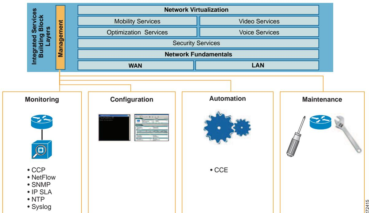
Cisco offers numerous tools for performing network management in the branch office. At this time, only a subset of those tools has been validated for the Streamlined Medium Branch Network. The primary focus was on monitoring the branch router. Future updates to this guide will address configuration management, automation, and maintenance for all the branch network devices.
