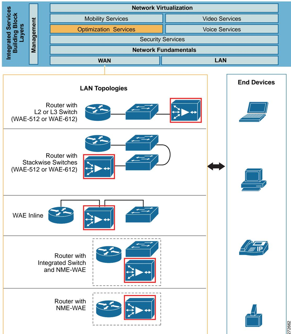
The Streamlined Medium Branch Network focuses on services that are integrated into the branch router. Designs featuring standalone Cisco WAE appliances are not considered in this guide. However, designs with standalone Cisco WAE appliances are equally viable and are described in the *Enterprise Branch Wide Area Application Services Design Guide* at:
