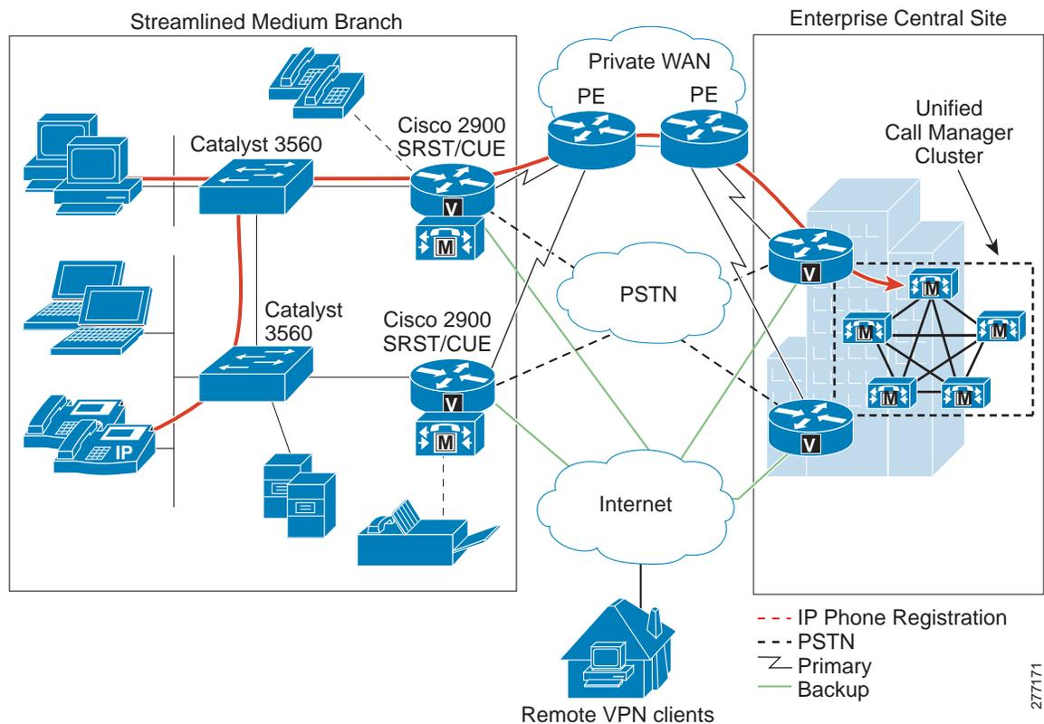
Under normal operations shown on the left in Figure 46, the branch office connects to the central site via a WAN, which carries data traffic, voice traffic, and call signaling. IP Phones at the branch exchange call signaling information with the Cisco Unified CM cluster at the central site. The voice gateway in the router forwards both types of traffic (call signaling and voice) transparently and has no “knowledge” of the IP Phones in the branch.
