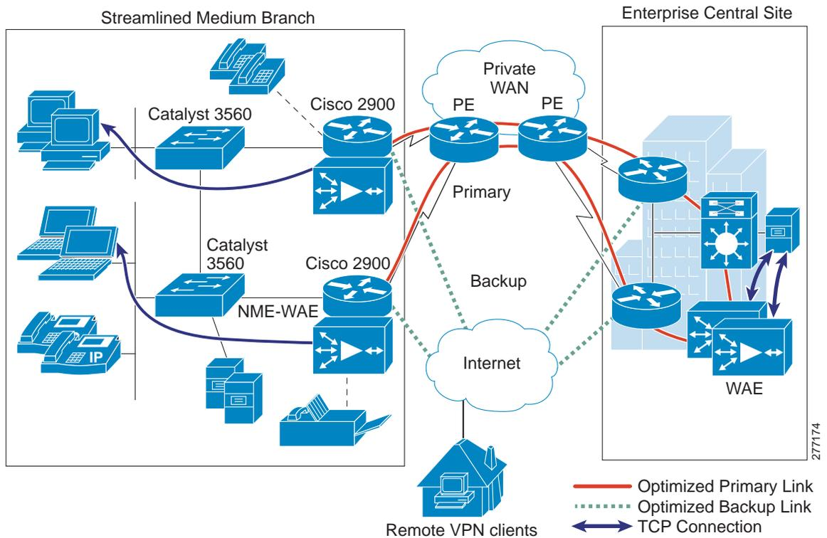
Cisco WAAS provides two options for controlling redirection and processing of application traffic:
