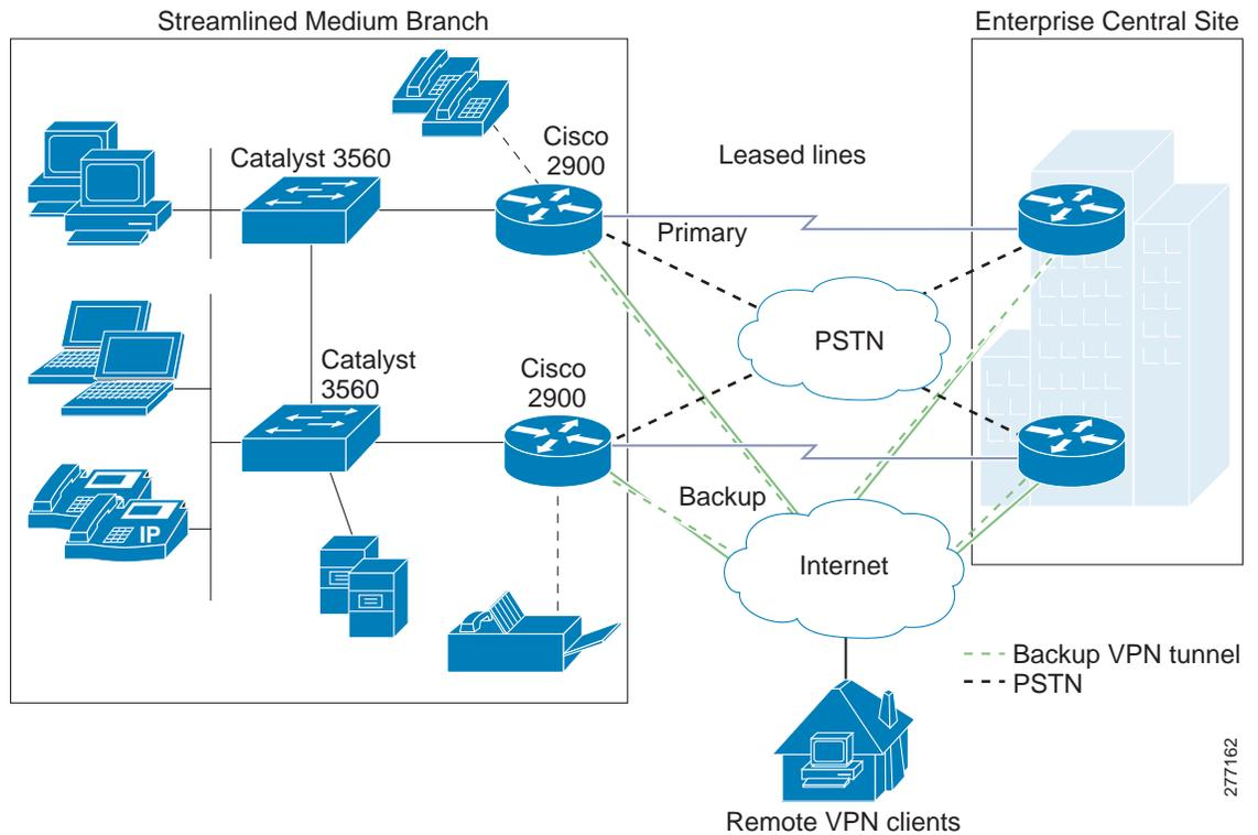
All traffic must be encapsulated by a data link layer protocol while it is crossing the WAN. The protocol defines how data is encapsulated into frames and the mechanism for transferring the frames between the branch and a central site. Selection of the data link layer protocol depends on the WAN technology and the communicating equipment in use. For leased-line WAN links, the following are the most prevalent data link protocols:
