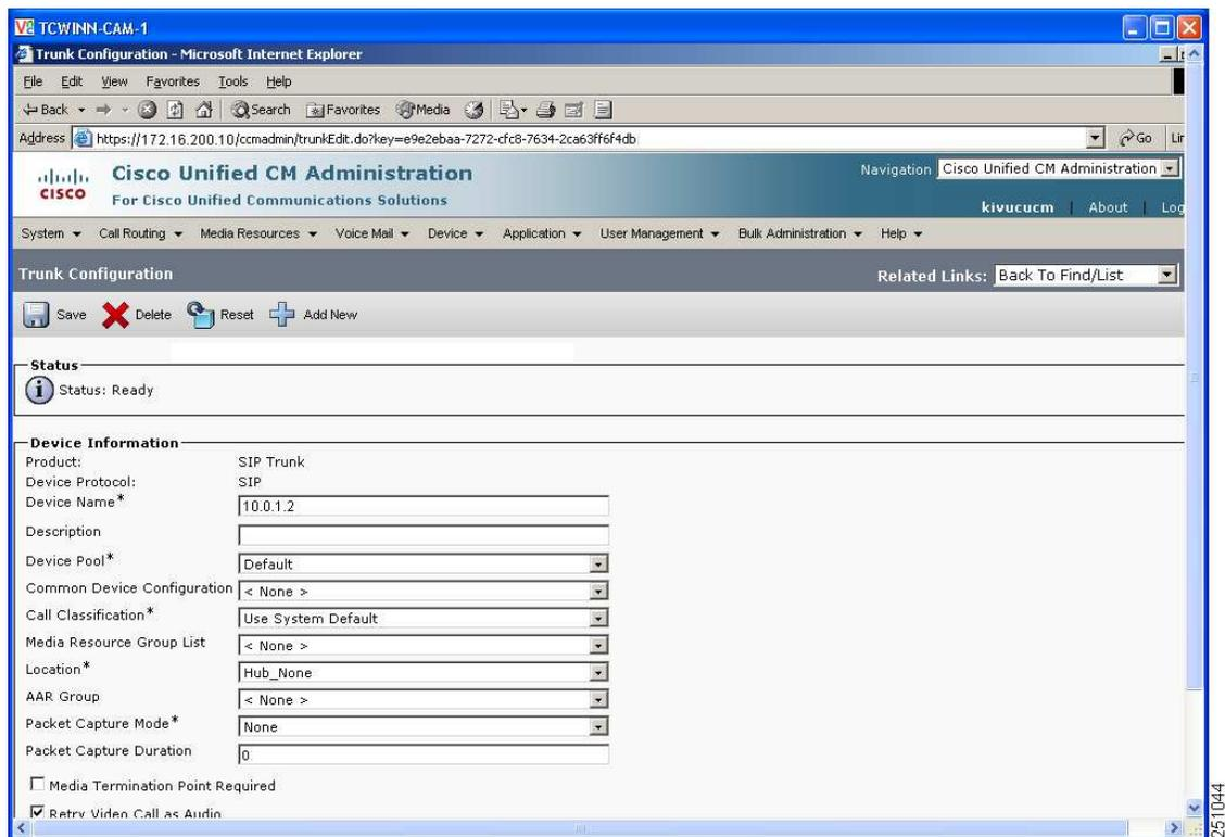
Figure 33 SIP Trunk Cisco Unified CM Configuration (2 of 3)
