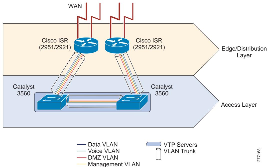
A switch can be configured as a VTP server, as a VTP client, or in transparent mode. A VTP server distributes and synchronizes VLAN information to VTP-enabled switches. VTP clients act on that information. VTP transparent switches are unaffected, but they pass VTP advertisements to other switches. The VTP domain delimits the portion of the LAN managed by a single VTP server.
