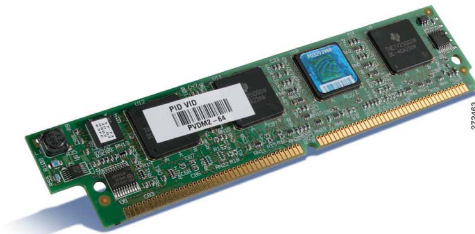
Figure 52 64-Channel Packet Fax/Voice DSP Module
