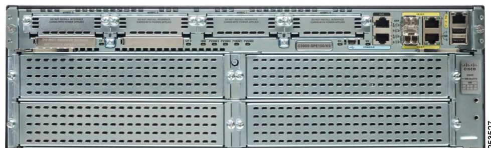
Figure 3 Interface Card and Service Module Configuration on a Cisco 3945 Router
