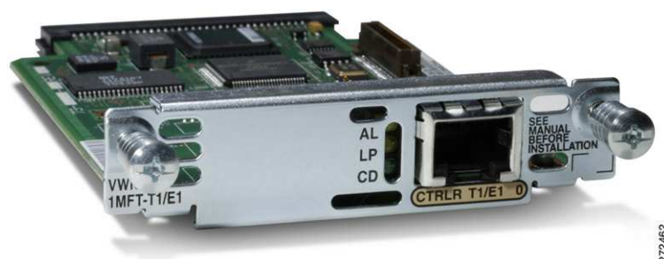
Figure 51 1 Port T1/E1 Multiflex Trunk Voice/WAN Interface Card
