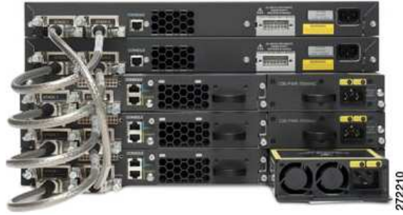
Figure 28 Catalyst 3750 in Cisco StackWise Configuration
