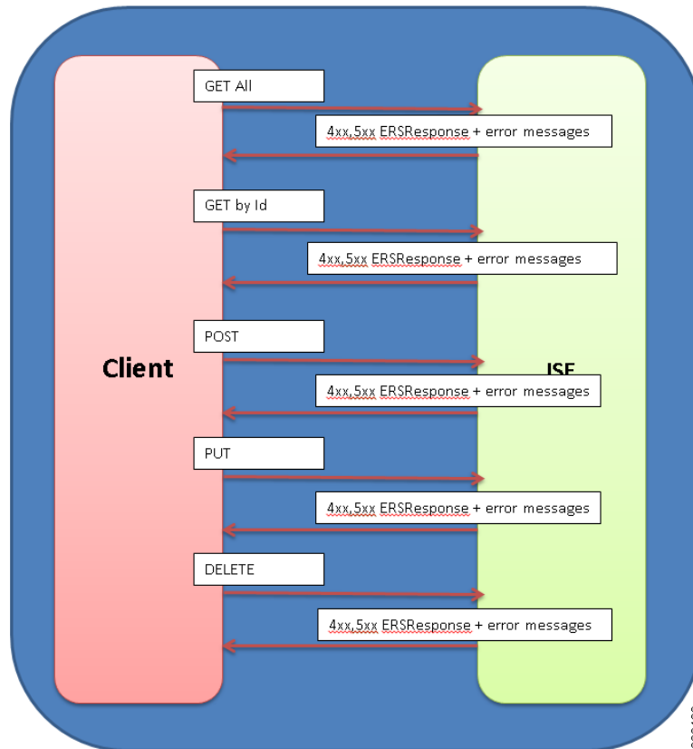
Figure 5-3 External RESTful Services Failure Flow Sequence
