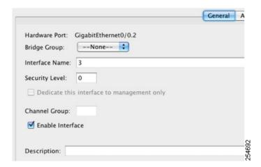
Do not use this procedure for Management interfaces; see the "Configuring a Management Interface (ASA 5510 and Higher)" section on page 18-11 to configure the Management interface.
