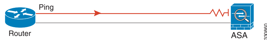
Figure 73-4 Ping Failure Because the ASA Has No Return Route
