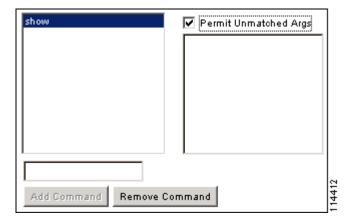
• For commands that are a single word, you *must* permit unmatched arguments, even if there are no arguments for the command, for example **enable** or **help** (see Figure 31-2).
