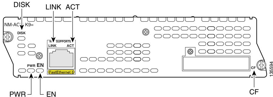
**Figure 2** NME-AON-K9= Faceplate
