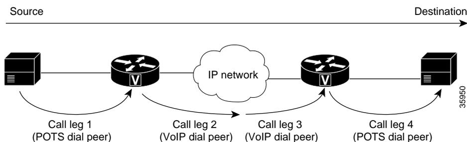
Legs connecting a local device (typically a phone, fax machine, or PBX) to a gateway are called *POTS* (plain old telephone service) legs. Legs connecting a gateway to the IP network are called *VoIP* legs. A POTS or VoIP leg is either *inbound* or *outbound*, from the perspective of the associated gateway.
