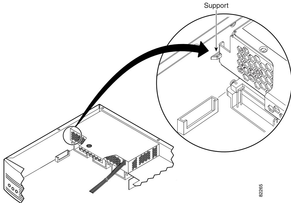
**Step 7** Pull the power supply back and lift the power supply out of the chassis. (See Figure 10.)
