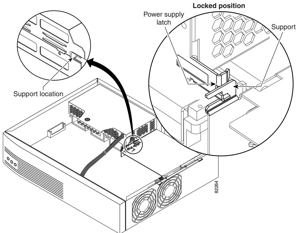
**Figure 9 Cisco 2691 Power Supply Mounting Support (Left)**
