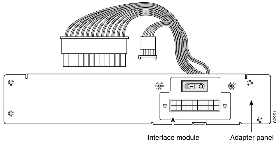
**Figure 2 Redundant Power Supply Interface Module Location in the Cisco 2691 Router**
