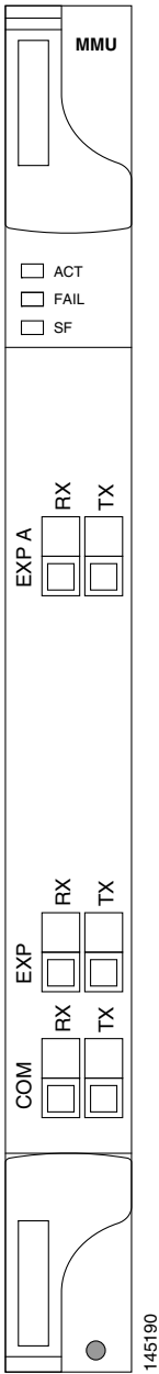
Figure 9-40 MMU Faceplate and Ports
