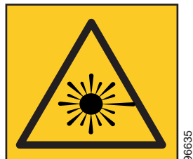
Figure 7-3 Laser Source Connector Label
