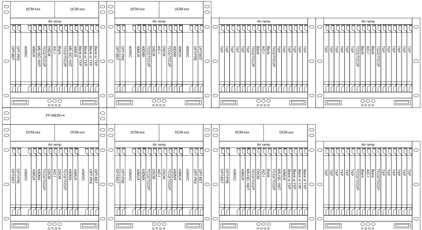
Figure 9-31 Four-Degree Protected Line Termination Mesh Node Layout
