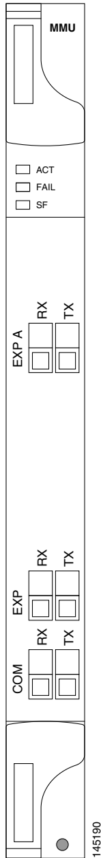
Figure 2-74 MMU Faceplate and Ports
