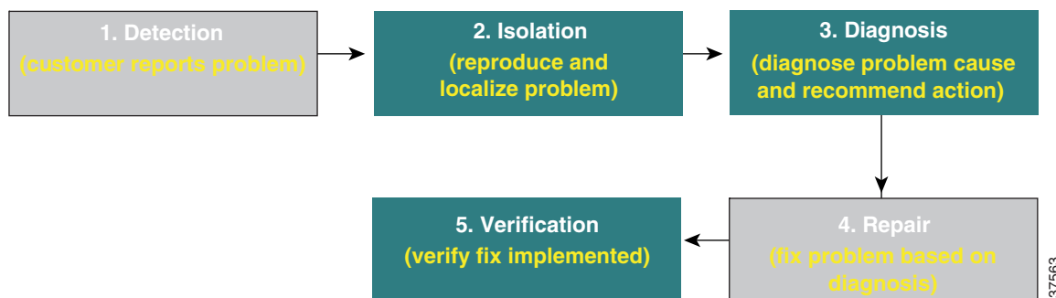
Figure 11-1 The Reactive Fault Lifecycle
