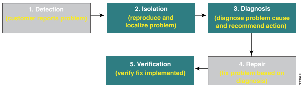
Figure 11-1 The Reactive Fault Lifecycle
