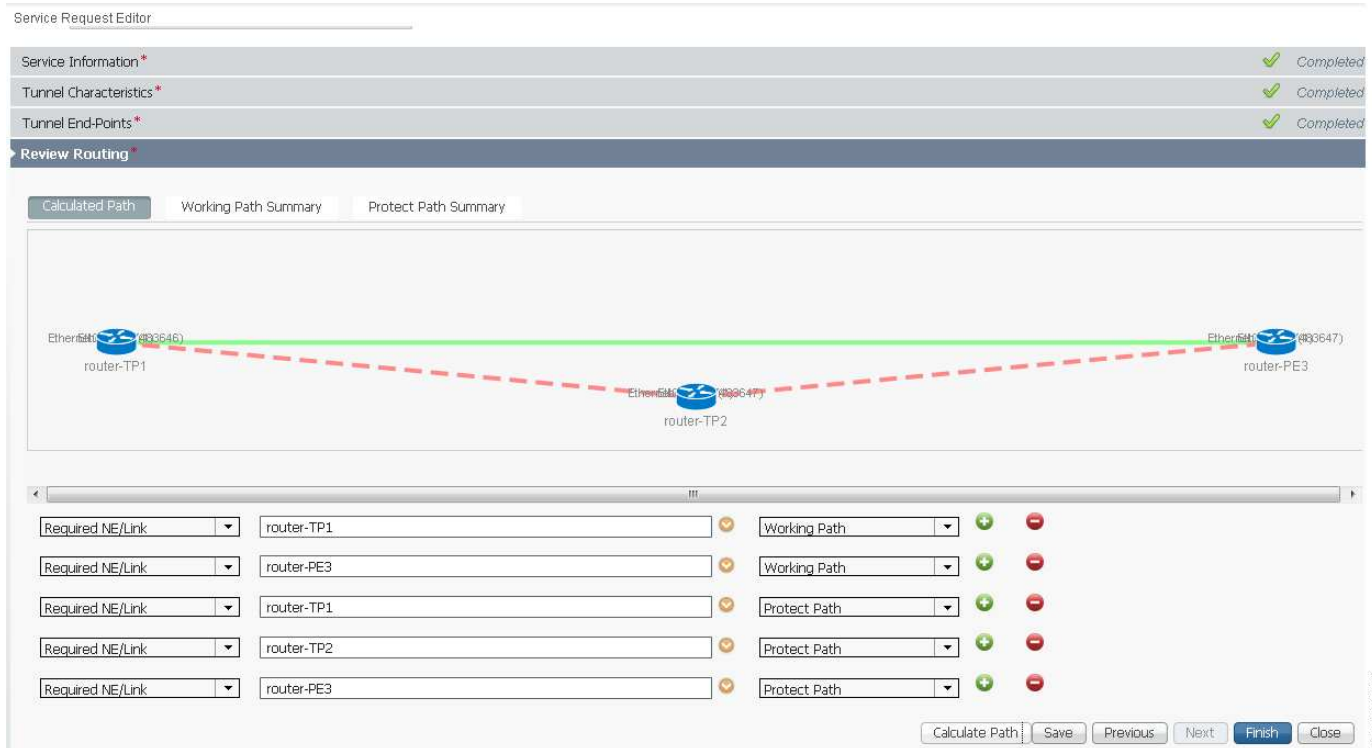
Figure 6-3 MPLS-TP Routing Diagram
