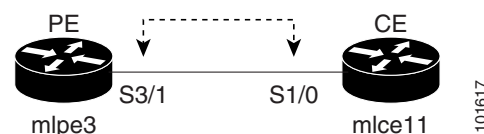
Figure 27-1 PE to CE link with CE Present
