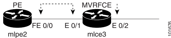
Figure 26-2 MVRFCE PE-CE Link with No CE
