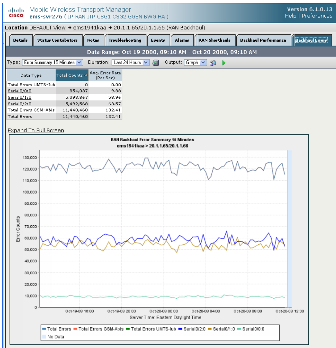
Figure 11-5 Example of Errors Tab for Backhaul Interface
